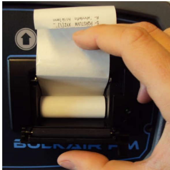
Figure 7 - Inserting Paper Roll
