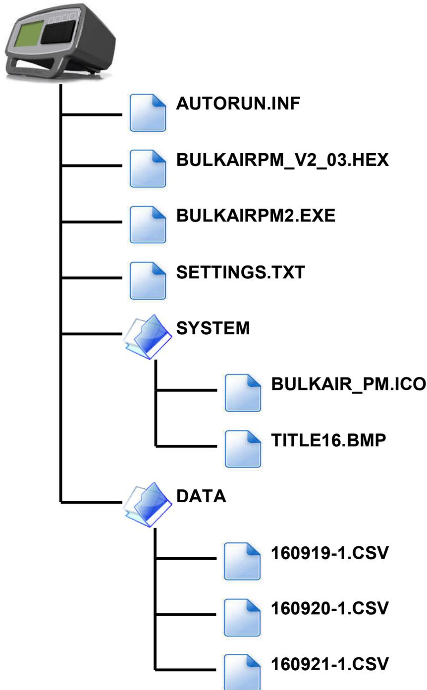
Figure 23 - Bulk Air PM SD Card Filing Structure
