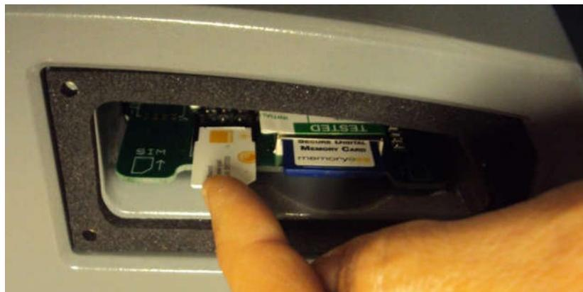
Figure 16 - Inserting the SIM Card
