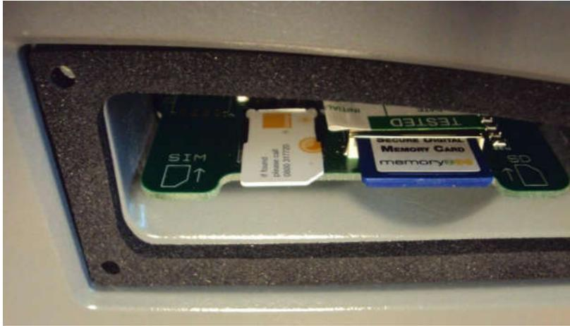
Figure 17 - SIM Card Fitted in Place
