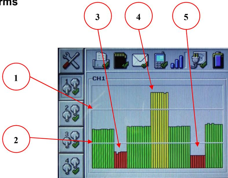
Figure 5- Alarm Activation (PRESSURE CHANNEL 1 SCREEN)
